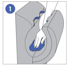
Wipe all surfaces with a soft cloth and non-abrasive cleaner. Particular attention should be paid to the seals and sides of the machine.
